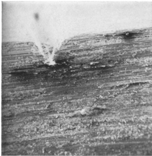
Figure 6 SE micrograph of the debonding zone at the instance of fracture initiation ( \times 40 ).
